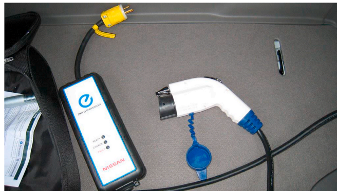
Fig. 19. An example of a Level 1 portable charger. "The 110/120V charging 'nozzle'" by Major Nelson is licensed under CC BY 2.0.
