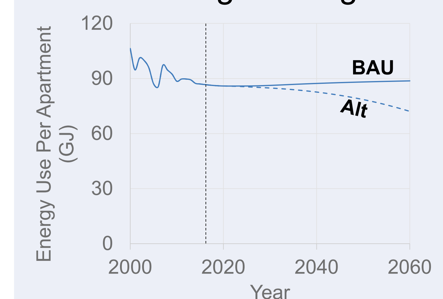
Fig. 6. Energy use per apartment per year. A 35% efficiency reduction of new apartments corresponds to a drop of 16.6 GJ per apartment by 2060.
